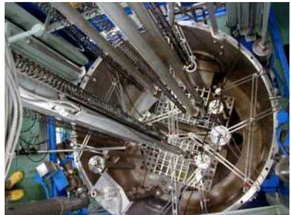
C frame: light water moderator frame
